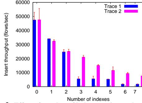
Figure 2: **Effect of number of indexes on insert throughput.** Indexes significantly cut throughput for both traces.
