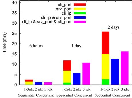
Figure 4: **Time to index the materialized view.** We are showing the time to create one through three indexes concurrently and compare it with the time to create them sequentially. Concurrent indexing is significantly faster than sequential indexing and it is little compared to view materialization.
