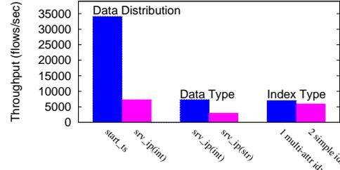
Figure 3: **Effect of type of indexed attribute on insert throughput.** The throughput of a database depends on the properties of the indexed attributes. `srv_ip(int)` represents a hash value of the string `srv_ip(str)` attribute.
