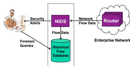
Figure 1: **Network intrusion detection system with a historical flow database.** The NIDS receives network flow summary data (such as NetFlow data [8]) from the enterprise’s internal routers, processes them, and generates alerts. While doing so, it maintains historical flow summary data for network forensic analysis.
