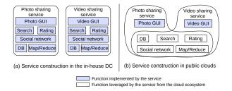
Figure 3: Simplifying Web service construction in public clouds. Web service construction in (a) in-house and (b) public-cloud environments. In the in-house datacenter, services cannot outsource their modules to other services over the WAN, leading to many services implementing entire software stacks redundantly. In public clouds, a Web service should be able to seamlessly leverage other services living in the cloud's ecosystem (e.g., media indexing and search, social networking data, etc.).
